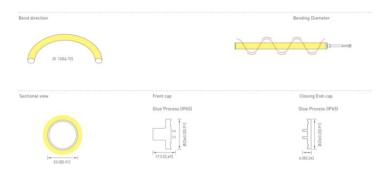
Remarks: "L" is the standard size of the light strip, can be customized according to the multiple of the minimum cutting unit length.
