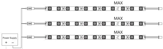
Note:the "MAX" here means the max connectable series
